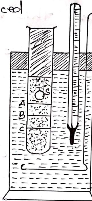
time of its falling through two successive equal distances AB and BC are noted. If they are equal, it means the sphere has acquired a constant velocity. If not, then other balls of smaller size are similarly examined. In this way a few balls are selected for each of which the time of fall through AB and BC is same. These balls are wetted thoroughly in the liquid. Now, one of them is dropped in the cylinder and the time taken in falling through the distance AB
